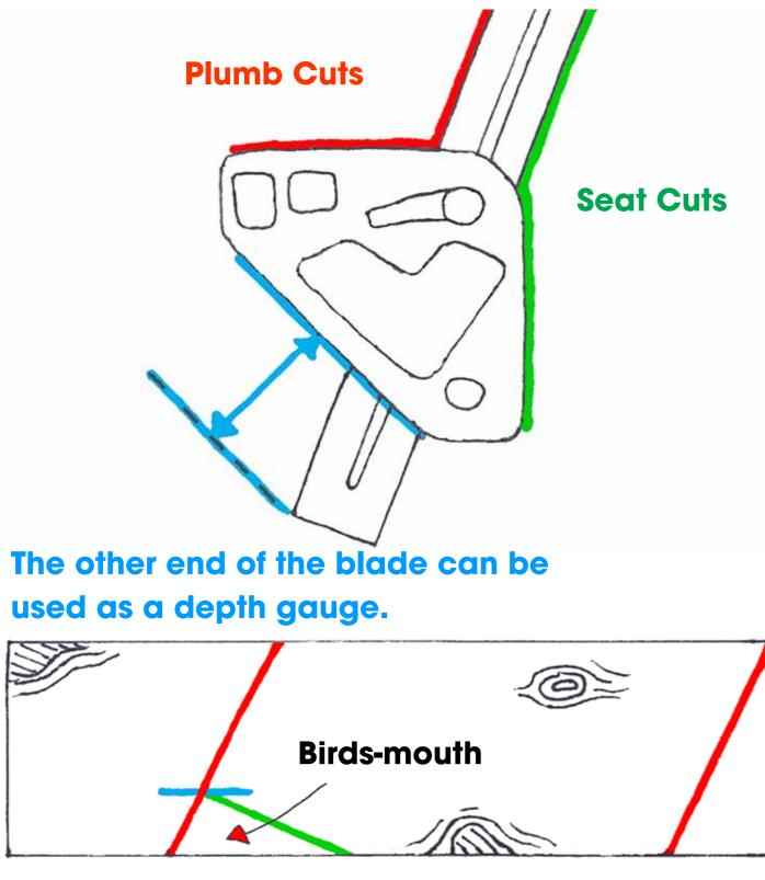
**Rafter cuts using the Primary Angle** Configuration.
